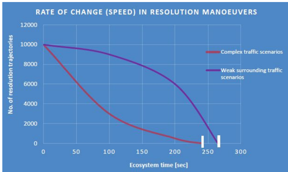
Figure 2-1: Perishable rate in the number of resolution maneuvers for two scenario types
