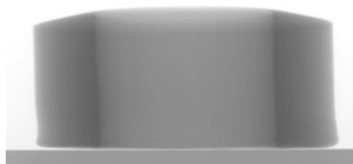
Figure 5.25 – X-ray image after the thermal treatment of 0.3\text{ }^{\circ}\text{C}\cdot\text{min}^{-1} until 200\text{ }^{\circ}\text{C} under \text{Ar}/5\%\text{H}_2 atmosphere.
