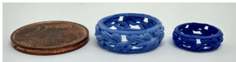
Figure 5.44 - Image of printed LTCC ring a) green body and b) sintered part.
