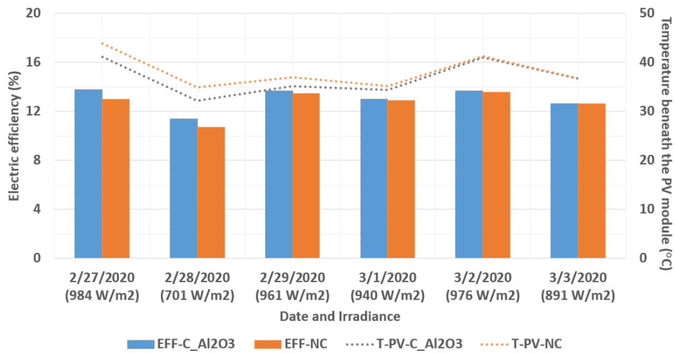
Figure 3-13. Variation of module temperature and electric efficiency of PV module with Al 2 O 3 coating and the no coating (NC) module in function of the solar radiation and coating days.
