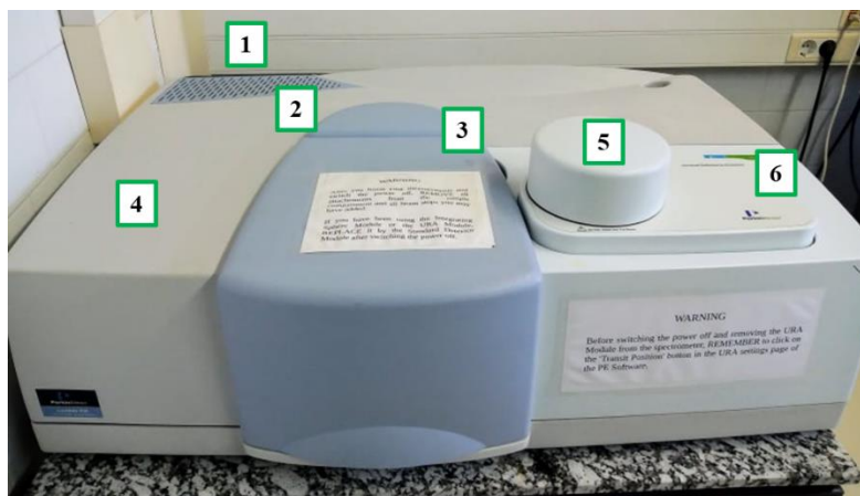
Figure 3.10: Perkin Elmer Lambda 950 model attached with a Universal Reflectance Attachment (URA) along with, 1) light source, 2) optical setup, 3) monochromator, 4) beam splitter, 5) sample stage, 6) detector. The arrow indicates the best possible movement of light from the power source to the detector.
