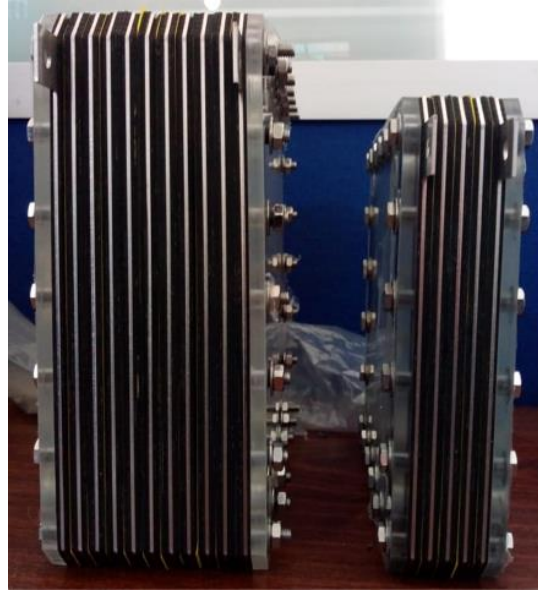
Figure 5-4: Alkaline electrolysis cells used in experimental tests
