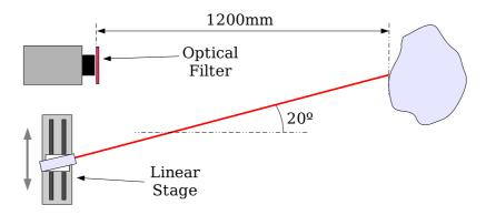
Figure 1.2: Set up of Forest's scanner
