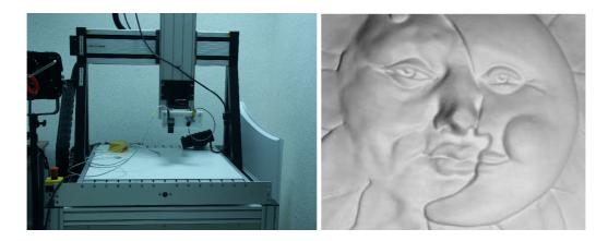
Figure 5.4: Set-up used in the experiments: a) Translation table and b) plaster object
