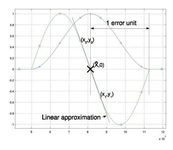
Figure 4.3: Use of zero crossing in the first derivative to determine laser peak position
