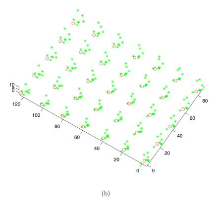
Figure 5.8: Results of the robot arm calibration: a) calibration pattern; b) 3D alignment of the calibration points where every cross represents the center of the circles computed in each acquisition and the dot represents the theoretical position of them
