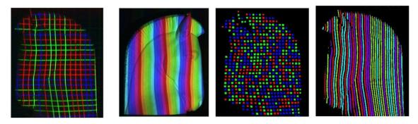
Figure 2.1: Some examples of coded structured light patterns
