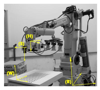
Figure 5.7: Industrial manipulator used in experiments. The four coordinate frames are represented: W (world), R (robot), H (Hand) and S(Scanner)
