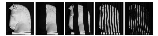
Figure 2.2: Sequence of patterns to code the scene
