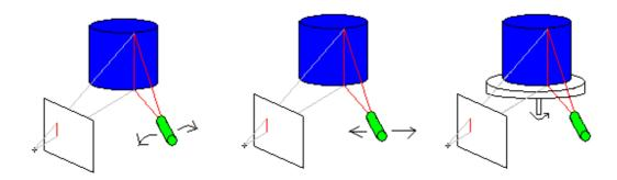
Figure 2.3: Examples of laser projection triangulation principle
