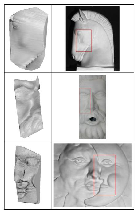
Figure 4.14: Set of acquisitions of the 3D hand-held sensor. Acquisitions of the left and real objects on the right. The box shows the acquired area
