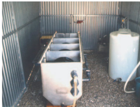
Figure 2.2 Pilot plant consisting of four biodiscs connected in series in Girona's wastewater treatment plant (Campdorà, NE Spain).
