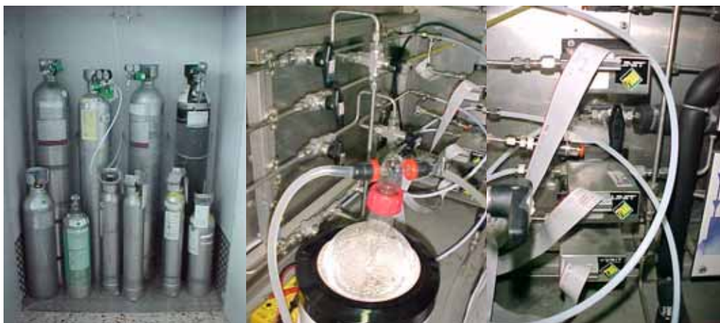
Figure V.21. Gas flow system: Gases stored in bottles under high pressure (left); Gas transport system (center); Mass-flow controllers (right)
