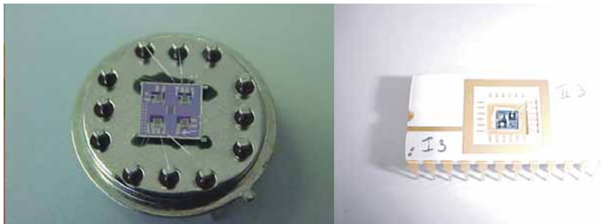
Figure V.7. Sensors bonded on different packages (from left to right: MHP, SOI)
