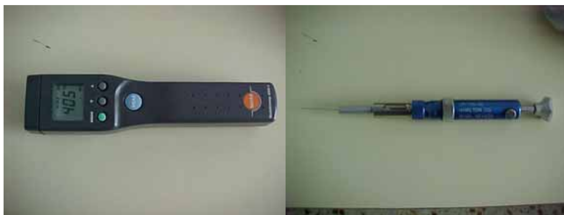
Figure IV.15. Devices used during the measurement: a) IR thermometer, b) High precision chromatographic syringe
