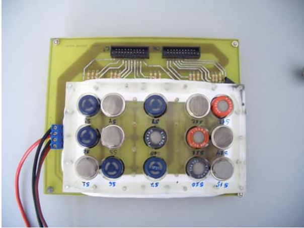
Figure 2: Sensor chamber, capacity 15 commercial sensors (FIS and taguchi TGS)
