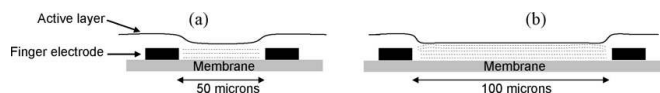
Fig. 5. Schematic illustrations of a cross section of the micro-sensor membrane for two fingers of the electrode. The current flow through the active layer is represented in dashed lines for the electrodes with narrow (a) and wide gap (b).
