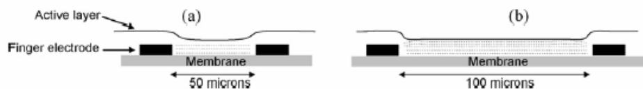
Figure 4.12. Schematic illustrations of a cross section of the micro-sensor membrane for two fingers of the electrode. The current flow through the active layer is represented in dashed lines for the electrodes with narrow (a) and wide gap (b).
