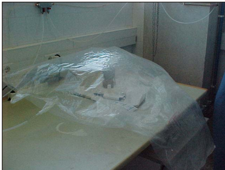
Figure II.10 Inflatable polyethylene chamber, Atmosbag, of Sigma-Aldrich
