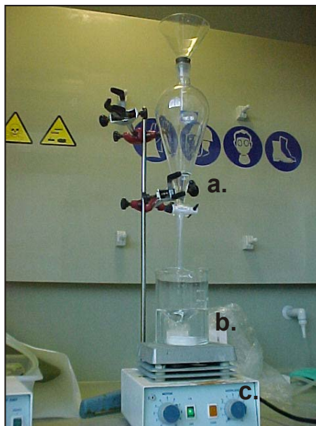
Figure II.11 a. 0.5 M solution of organic precursors in isopropanol b. Acid solution under stirring c. Stirring machine
