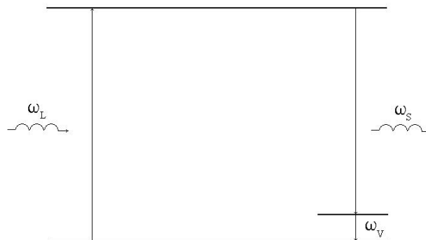
Fig. 2.1. Schematic diagram of Raman scattering.
