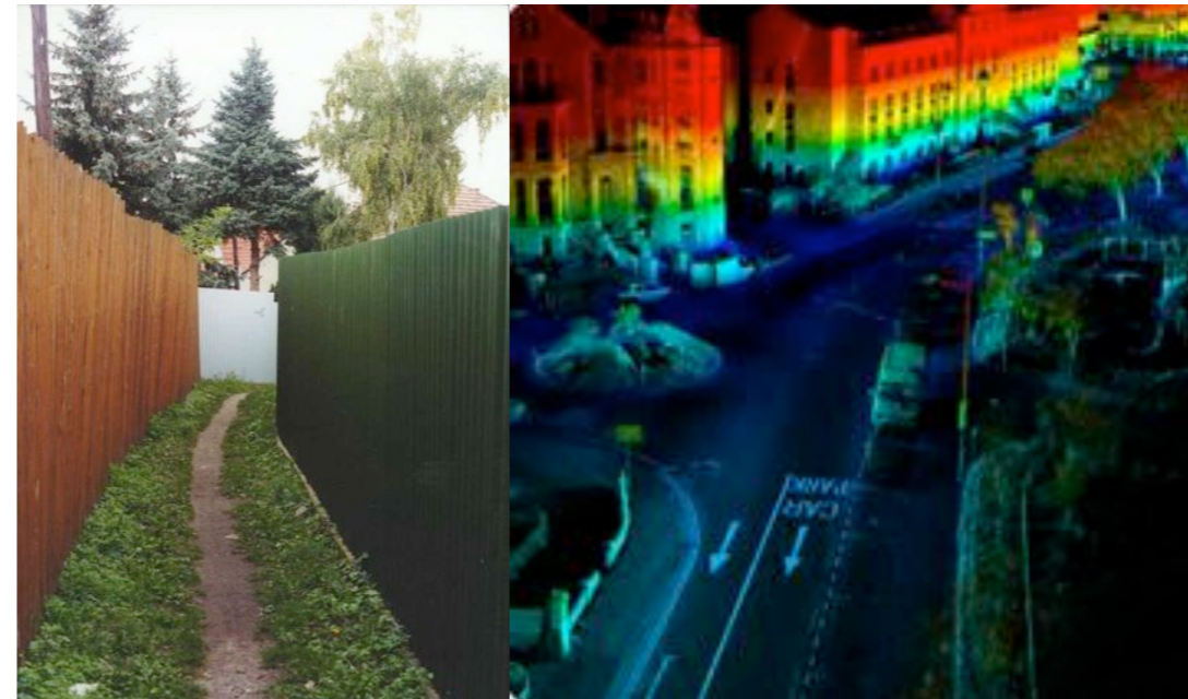
Figure IV.50: Left: suburban residential neighbourhood in Bratislava (Slovak Republic), 2002: private territories extracted from visual scope. right: urban mapping based on maximum visual scope of LIDAR technology (Light Detection and Ranging), an optical remote sensing technology that measures properties of scattered light to find range and/or other information of a distant target.
