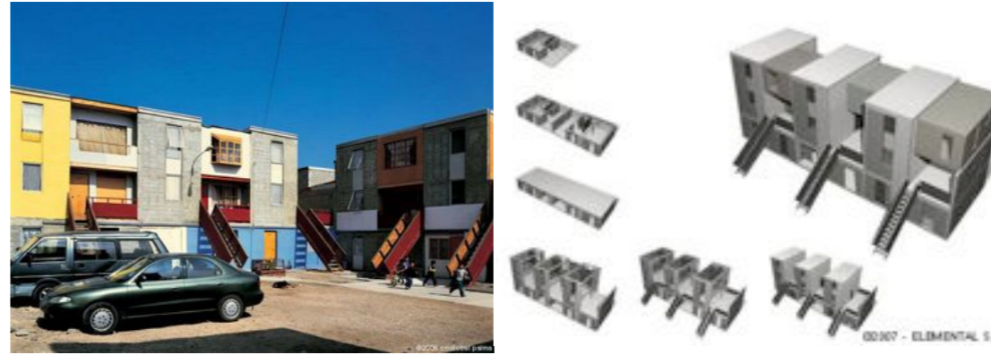
Figure IV.13: Iquique residential project (Chile), Alejandro Aravena, 2003-2004: shared courtyards give access to individual dwellings (original images from http://www.elementalchile.cl/category/vivienda/iquique/ )
