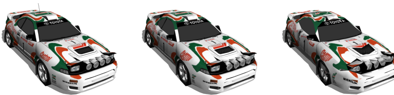
(c) Racing car model. From left to right: original (8,345 triangles), 66 % (5,506 triangles) and 33 % (2,753 triangles) version.
