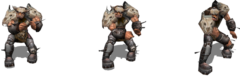
(a) Ogre model. From left to right: original (1,960 triangles), 66 % (1,292 triangles) and 33 % (646 triangles) version.
