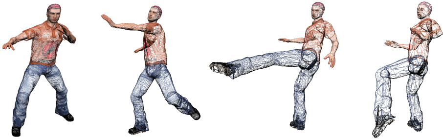
Figure 5.1: Approximations of a man model (136,410 triangles). From left to right: original model and simplifications to 50%, 25% and 10% respectively.
