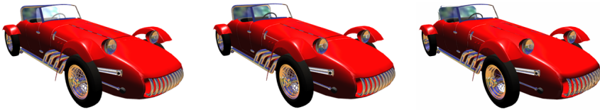
(b) Buggy model. From left to right: original (91,949 triangles), 66 % (60,686 triangles) and 33 % (30,356 triangles) version.
