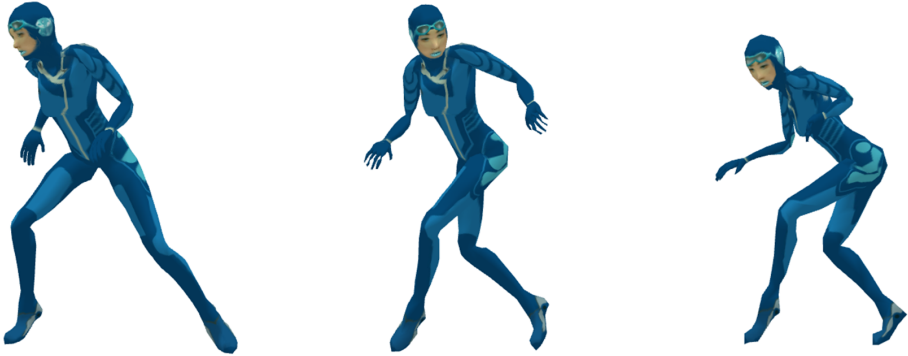
Figure 4.1: Space woman model. From left to right: original (4,130 triangles), 60 % (2,478 triangles) and 20 % (826 triangles) approximations.
