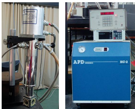
Figure 4.10: Closed-cycle helium cryostat components (left) and compressor (right) used for low temperature experiments down to 15 K.
