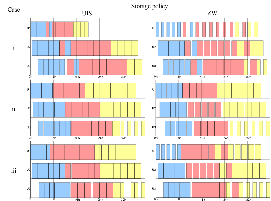
Figure 8.3: Gantt Charts obtained for scenario 2 in Example 2. (Product 1 in yellow, Product 2 in red, and Product 3 in blue)
