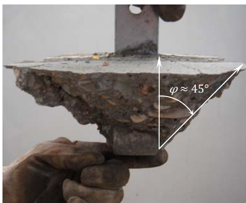
Fig. 11. Failure conical shape for the PUC4 specimens.
