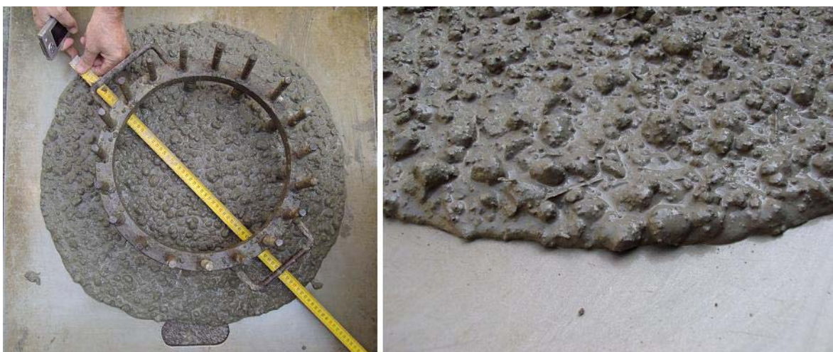
Fig. 10. Slump flow test with the Japanese ring and the edge of concrete, concrete P 9 .
