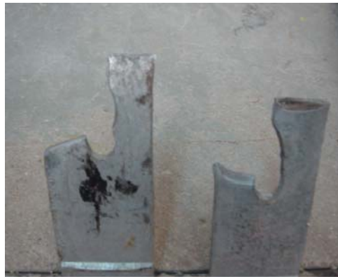
Fig. 9. Failure of the strip due to an inappropriate connection.
