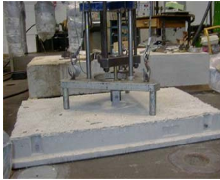
Fig. 2. Anchor pullout test set-up from IETcc.
