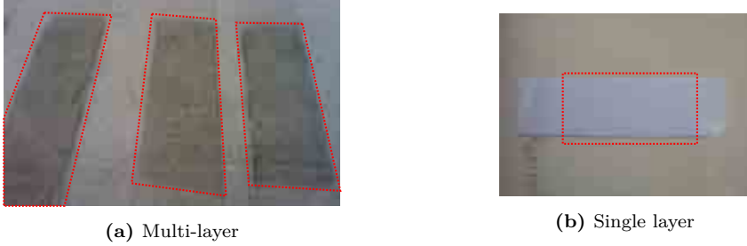
Figure E.7: Samples of (a) multi-layer and (b) single layer graphene. The dashed red frames mark the region occupied by graphene, where the multi-layer samples can be easily spotted thanks to the higher attenuation at optical frequencies versus the single layer sample.
