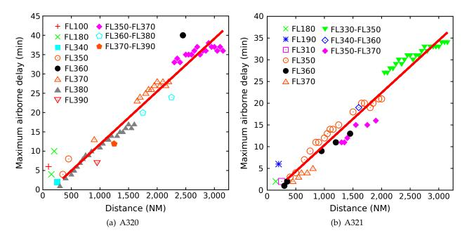
**Figure IV-10:** Airborne delay and optimal flight level as a function of flight plan distance for A320 and A321 aircraft types
