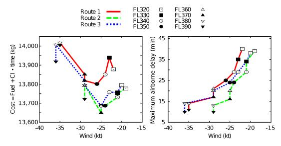
Figure IV-16: Optimal flight level, cost and maximum airborne delay as a function of route for Orlando International to Chicago O'Hare flights
