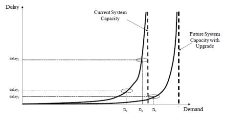
Figure I-2: Relationship between delay, demand and system capacity Source: (Ball et al., 2010b)
