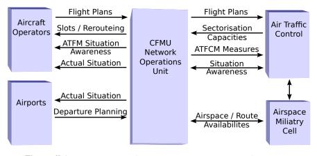
Figure II-3: CFMU network operations unit operational structure. Based on: (Eurocontrol Central Flow Management Unit, 2011).
