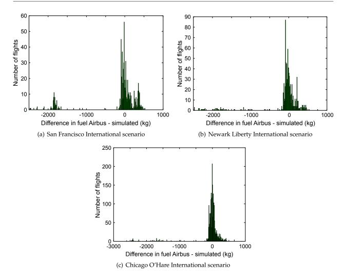
Figure C-1: Difference in total fuel burnt between Airbus PEP computation and simulation
