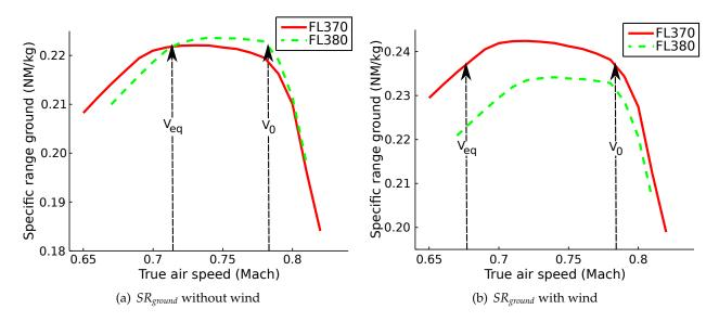
**Figure III-17:** Effects of wind on the optimal flight level and in the margins between  $V_0$  and  $V_{eq}$  speeds
