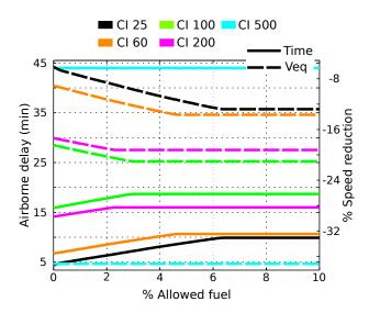
**Figure IV-25:** Airborne delay and speed reduction for the Frankfurt to Madrid route as a function of the extra fuel allowance
