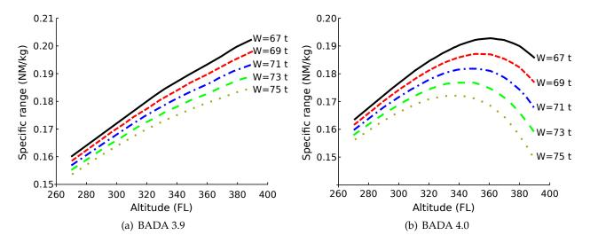
Figure B-3: Specific range as a function of altitude for typical twin engine aircraft at M0.78 Based on: (Poles et al., 2010)
