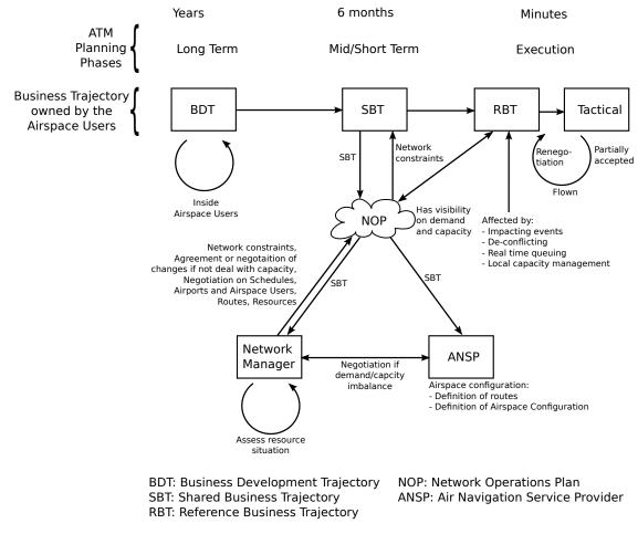
Figure II-5: Trajectory development under SESAR concept of operations.
