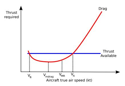
Figure III-5: Thrust required and available curve
