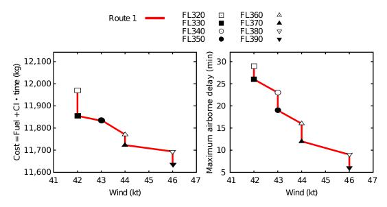
Figure IV-17: Optimal flight level, cost and maximum airborne delay as a function of route for Austin-Bergstrom International to Chicago O'Hare flight
