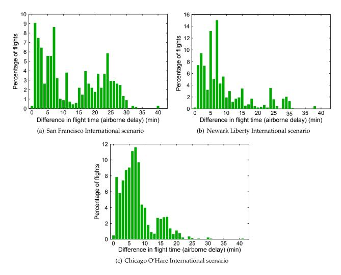
**Figure IV-8:** Difference in flight time (airborne delay) between the simulated nominal flight and the speed reduction flight
