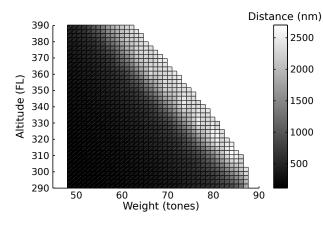
Figure III-14: Distance needed to absorb 10 minutes of delay without extra fuel burned
