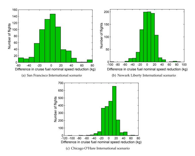
Figure C-5: Difference in cruise fuel between simulated nominal flight and speed reduction flight
