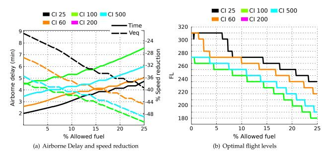
**Figure IV-27:** Airborne delay, speed reduction and flight level for the Dublin to London Heathrow route as a function of the extra fuel allowance
