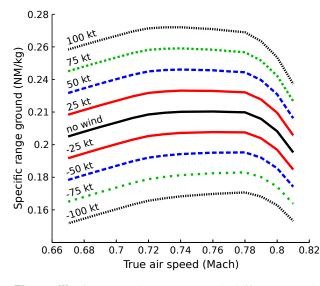
Figure III-16: Typical SR curve with different winds
