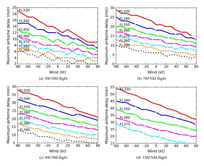
**Figure IV-14:** *Maximum airborne delay as a function of flight level and wind (constant wind during the cruise)*
