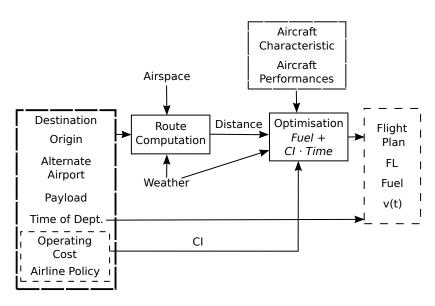
**Figure III-2:** Scheme of the current flight optimisation ( $J = Fuel + CI \cdot Time$ ) realised by aircraft operators
