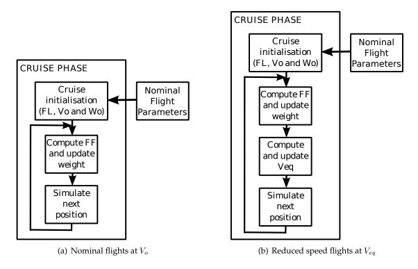
Figure IV-5: Diagram of the flight simulation in FACET
