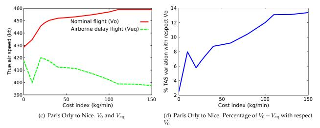
**Figure III-18:** Margin between  $V_0$  and  $V_{eq}$  as function of CI in calm wind scenario
