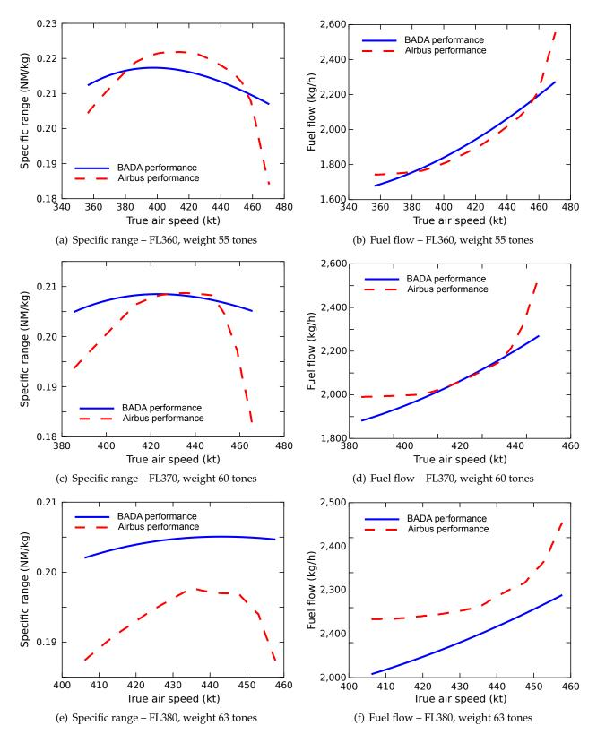
**Figure B-1:** Medium size twin jet engine Airbus model. BADA and PEP performances comparison as a function of cruise speed
