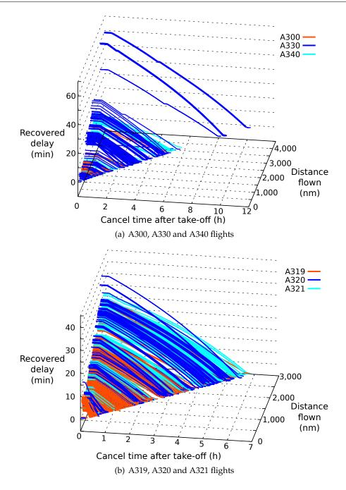
**Figure IV-9:** Potential delay recovered as a function of flight time and the length of the flight plan for flights with destination EWR, ORD and SFO
