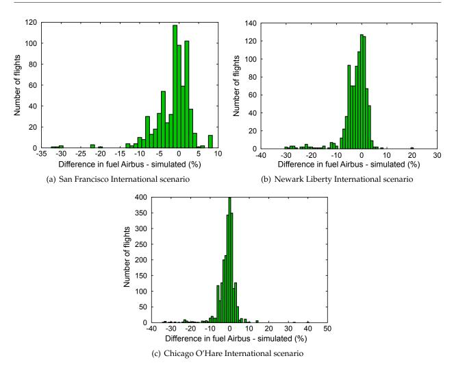
**Figure C-2:** Difference in total fuel burnt between Airbus PEP computation and simulation in percentage with respect Airbus fuel
