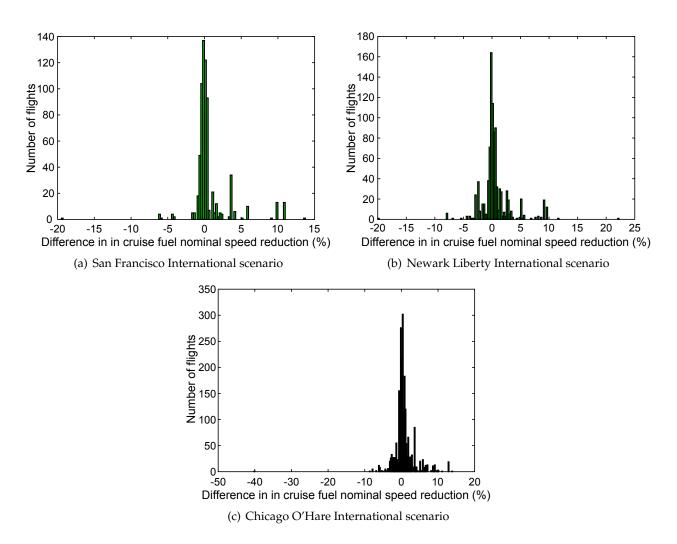
**Figure C-4:** Difference in cruise fuel between simulated nominal flight and speed reduction flight in percentage with respect nominal flight
