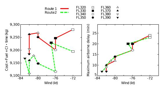
**Figure IV-18:** Optimal flight level, cost and maximum airborne delay as a function of route for Washington Dulles International to Chicago O'Hare flight
