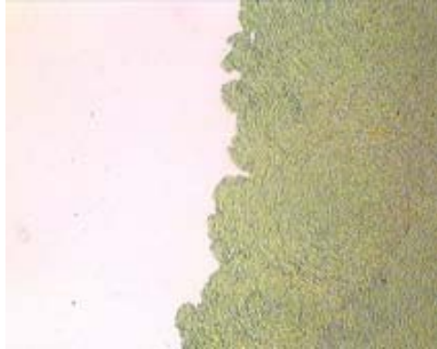
Figure 5.3: The image was taken with an optical microscope showing the visible degradation of the sample surface when capped with 10nm Mg and 20nm Pd layer.
