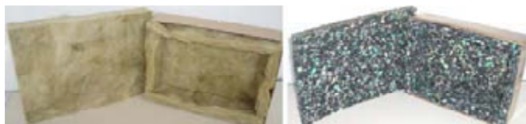
Figure 2. Cardboard boxes and their lids covered with glass wool and polyurethane foam, respectively.
