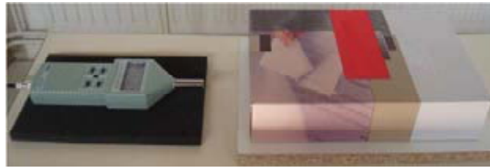
Figure 5. Experiment to test the capacity of sound attenuation produced by the material inside the box.
