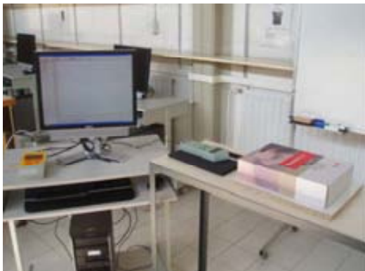
Fig. 2 Experimental setup (sound level meter-MBL interface-computer, box and lid covered with a certain material, buzzer inside the box)
