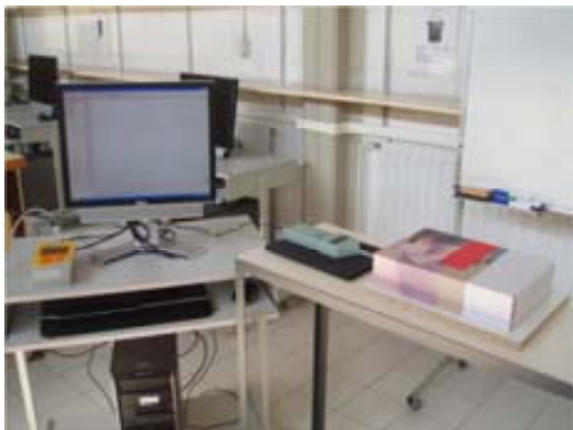
Figure 3. Experimental setup (sound level meter-MBL interface-computer, box and lid covered with chipboard-Formica, buzzer inside the box).
