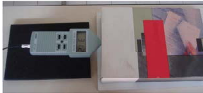
Figure 6. Experiment to determine the acoustic behaviour of the material inside the box.
