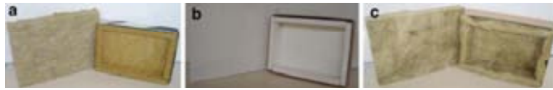
Fig. 1 Cardboard boxes and their lids covered with rock wool, expanded polystyrene and glass wool, respectively
