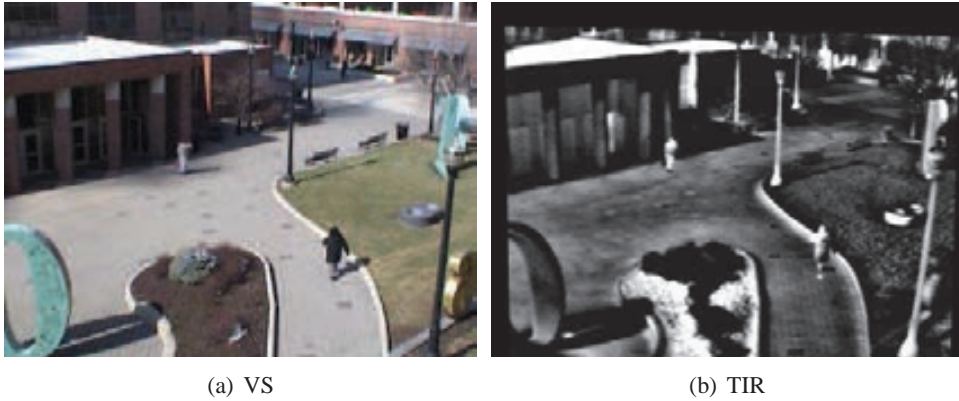
Figure 2.2: Out-door scene during daytime. (a) using a VS camera sensor, and (b) using a TIR camera sensor (images from [12]).
