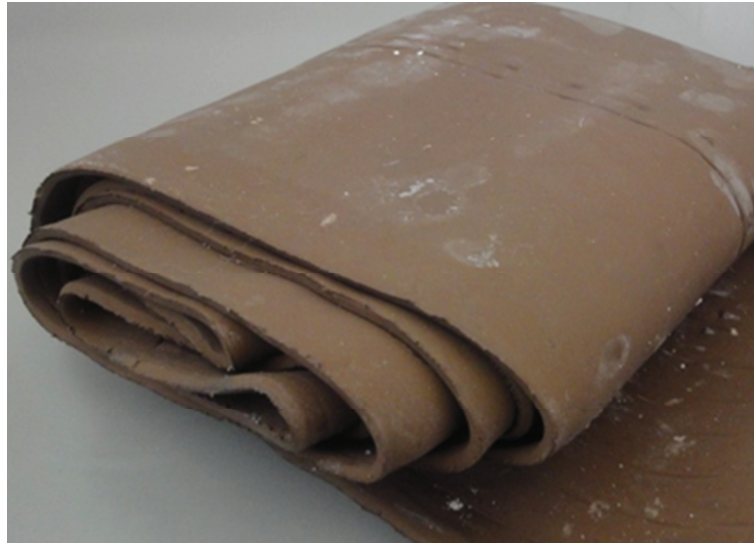
Figure 13. Composite dense sheet based on polymeric matrix incorporating PCM and EAFD.
