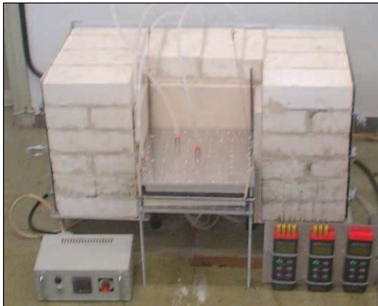
Figure 19. Conductimeter device: cold plate, data-loggers, insulation, and energy supply.
