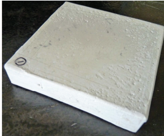
Figure 18. Samples analyzed in this study (in this case, gypsum + microencapsulated PCM samples).
