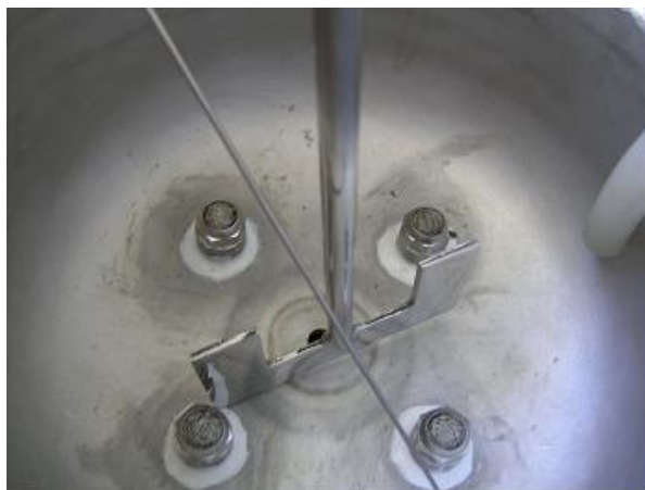
Figure 3.14. Aeration and mixing system in autothermal reactor
