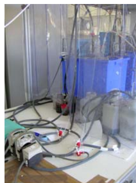
Figure 3.5. Sludge feeding and sample extraction
