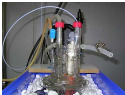
Figure 3.4. Cap reactor detail
