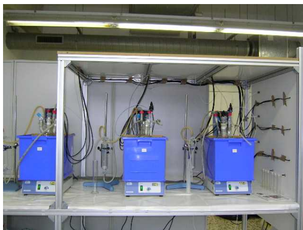
Figure 3.3: Anaerobic digestion pilot-plant
