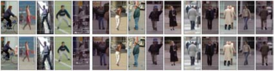
Figure 5.5: Alignment comparison between detections and annotations. Ground truth (top row) and detections (bottom row). Left block of five pedestrians contains detections with classifier score in [-1, 0) , those in mid block are in [0, 1) , and those in right block correspond to values \geq 1 . In our current settings, left and mid blocks are discarded and only the detections of the right block would arrive to the human oracle for validation (along with some hard negatives).
