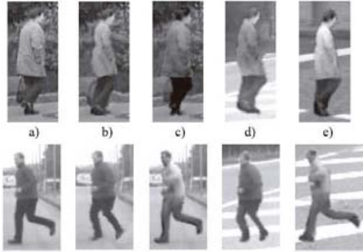
Figure 2.5: Example of virtual pedestrian synthesis from [32] original pedestrian examples, b) shape variation, c) foreground texture variation, d) - e) joint variation of shape, foreground and back-ground texture.
