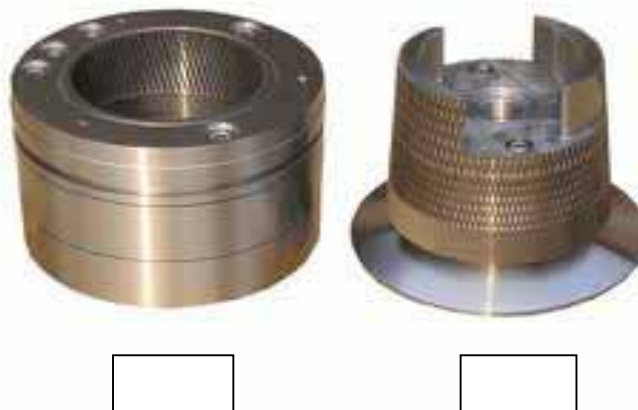
Figure 9. The two principle parts of the colloidal mill system
