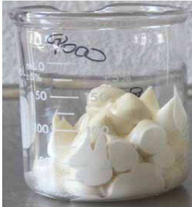
Figure 42. Emulsions containing 50% oil and 5% sodium caseinate after treatment by ultra-high pressure homogenization.
