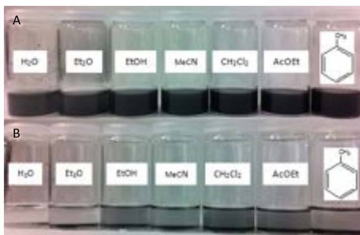
Figure 3.12. Dispersibility of rCNT-ppPFM in different solvents. Images of (A) right after sonication and (B) after settling at room temperature for 1 h.
