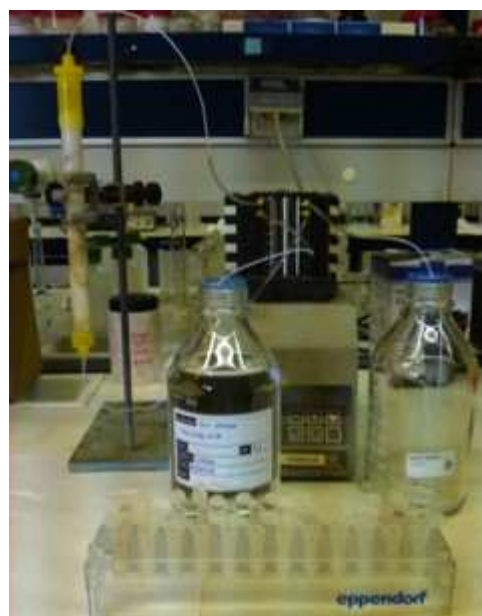
Figure 2.17. Experimental set-up of As(V) adsorption in continuous mode by gravity (a) and counterflow (b) for SPION loaded HPAN nanofibers with 20x1.5 cm columns
