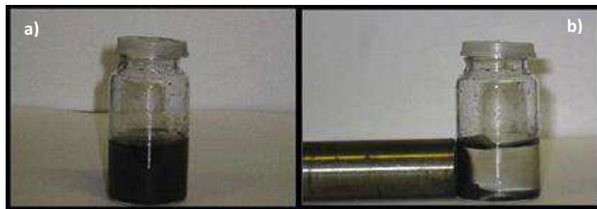
Figure 3.4. SPION suspension in TMAOH (a) and SPION separation from the solution under an external magnetic field (b).
