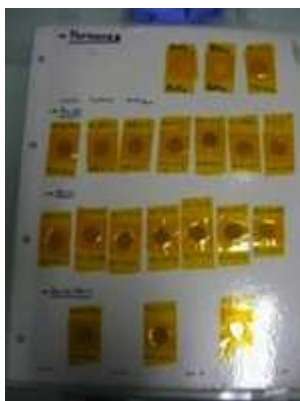
Figure 2.3. Example of pellet samples encapsulated in Kapton® foils for the synchrotron experiments.
