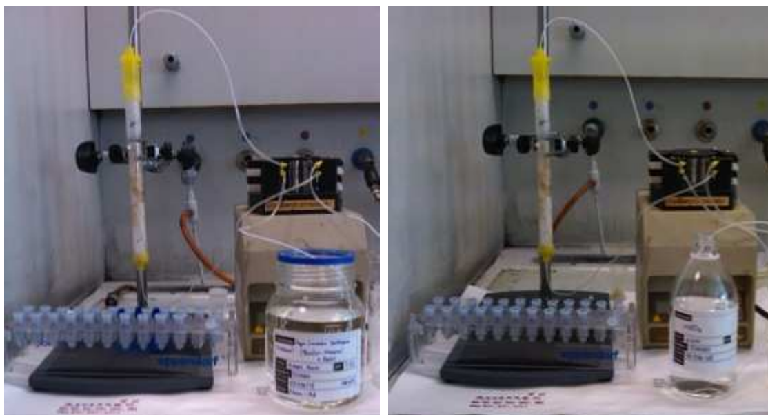
Figure 2.18. Experimental set-up of As(V) adsorption (a) and desorption (b) in continuous mode by counterflow with 20x1.5 cm columns
