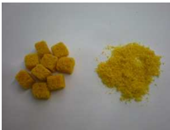
Figure 2.9. Forager® Sponge in cubic and dust form after milling
