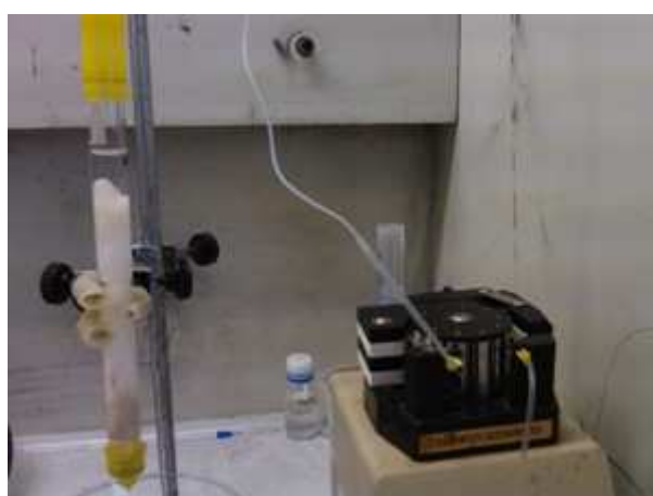
Figure 2.17. Experimental set-up of As(V) adsorption in continuous mode by gravity (a) and counterflow (b) for SPION loaded HPAN nanofibers with 20x1.5 cm columns
