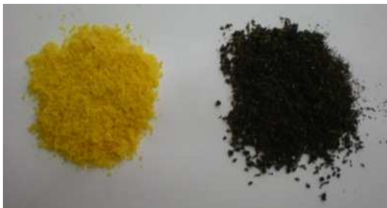
Figure 2.11. Forager® Sponge before and after the SPION fixation
