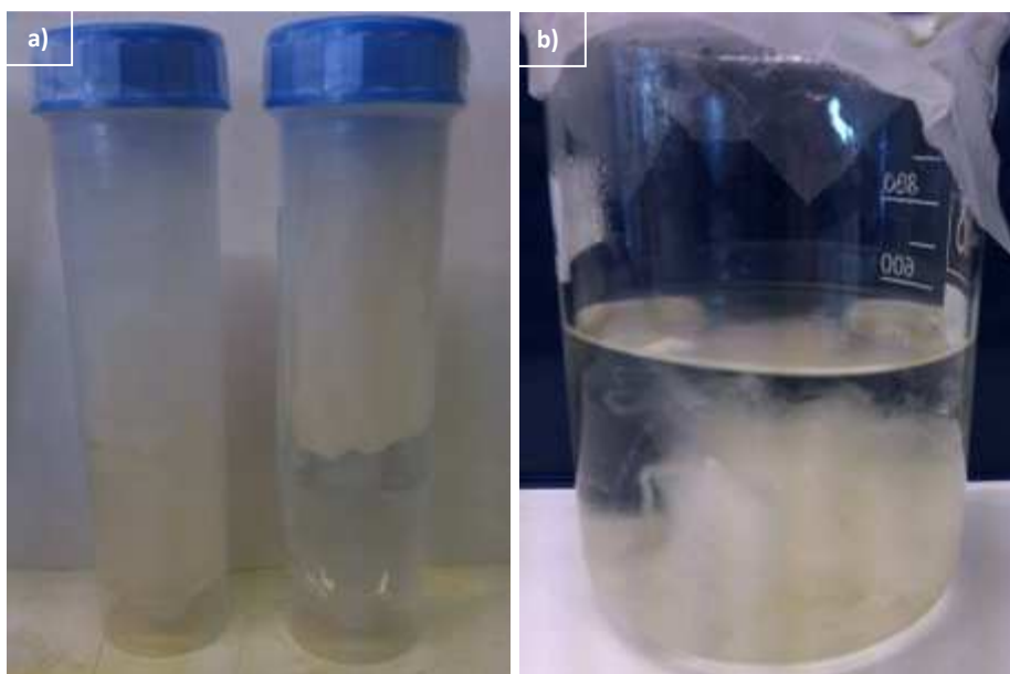
Figure 3.46. SPION loaded HPAN nanofibers after the SPION impregnation (a) and SPION loaded HPAN nanofibers 2 hours later in a water solution.
