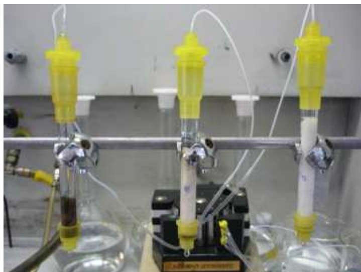
Figure 2.16. Experimental set-up of As(V) adsorption in continuous mode by gravity with 10x1.0 cm columns
