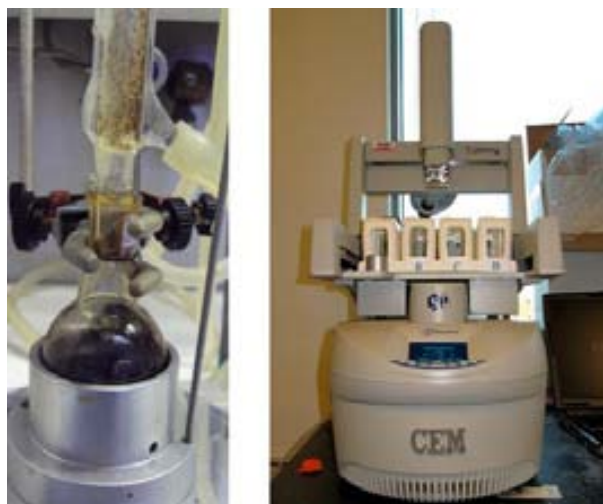
Figure 5.1.1.2: Pictures corresponding to a reflux setup (left) and a microwave device (right) used to carry on the different nanoparticles’ synthesis.
