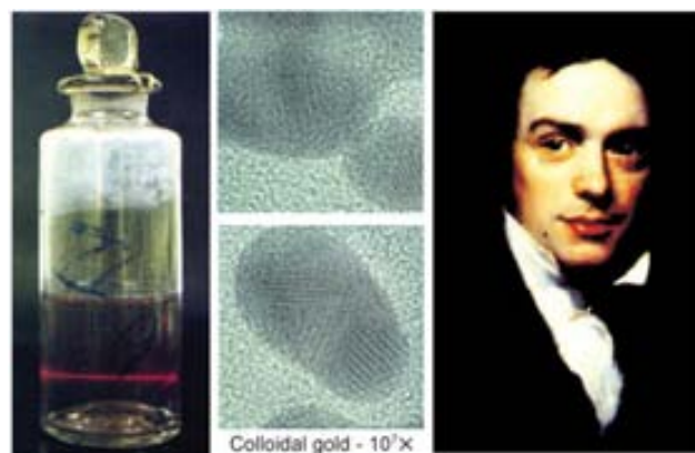
Figure 1.1.2: Faraday's gold nanoparticle dispersion (left), TEM image from this nanoparticles (middle) and Faraday's portrait (right)
