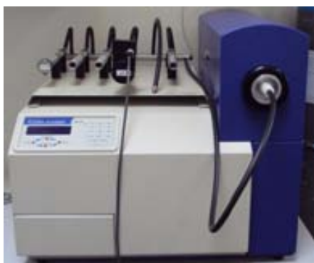
Figure 2.3.1.8: Picture of the plasma cleaner used to clean the surface of all the specimens analyzed via TEM .
