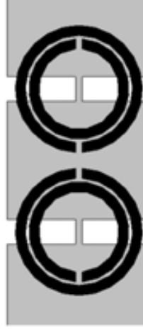
Figure 2.8. Typical layout of a CRLH SRR-based unit cell in CPW technology. The SRRs are etched in the back substrate side and the CPW is loaded with shunt inductances. Figure extracted from [37].
