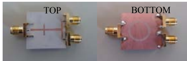
Figure 5.6. Schematic and photograph of the fabricated dual-band power divider.
