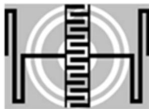
Figure 3.5. Topology of the unit cell of CSR-loaded CRLH microstrip lines. Figure extracted from [59].
