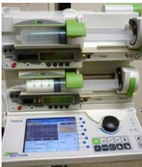
Figure 5-17: Drug infusion system available at the Chirurgische Universitätsklinik of the Homburg Hospital: two target-controlled infusion (TCI) integrated into a Workstation.
