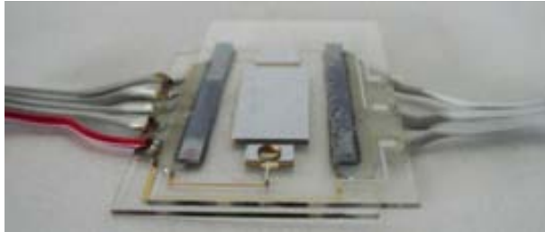
Figure 4-18: p-FAIMS device in the GL-Si-GL configuration with electrical wires.
