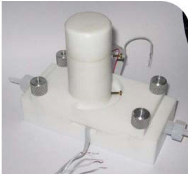
Figure 4-19: Packaging of the p-FAIMS device in the GL-Si-GL configuration with mechanized Teflon®.
