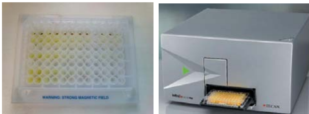
Figure 4.1 Polypropylene microtiter plate placed on the magnet for the capture of the magnetic particles before transferring the supernatants to the polystyrene plates for the final read-out (A) and image of a microplate reader used for the optical detection (B).
