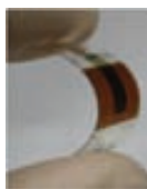
Figure 4.27 Photo of a flexible OSC with V_2O_5 \cdot 0.5H_2O as hole-transport layer.
