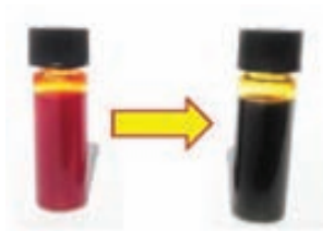
Figure 4.13 Appearance of a fresh V_2O_5 : IPA solution (left) and aged solution (48 hrs) (right)
