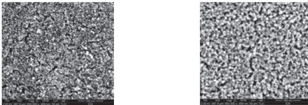
Figure 3.34 SEM images of ZnO-CBO (left) sample and ZnO, IPA sample (right)
