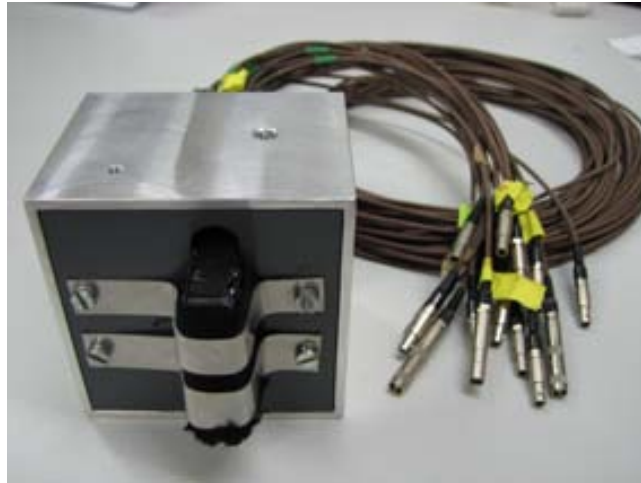
Figure 7.9: Single LYSO crystal and MCP-PMT mounted in an aluminum box for testing. Each of the 16 anodes illuminated by the crystal have been routed to a coaxial cable.
