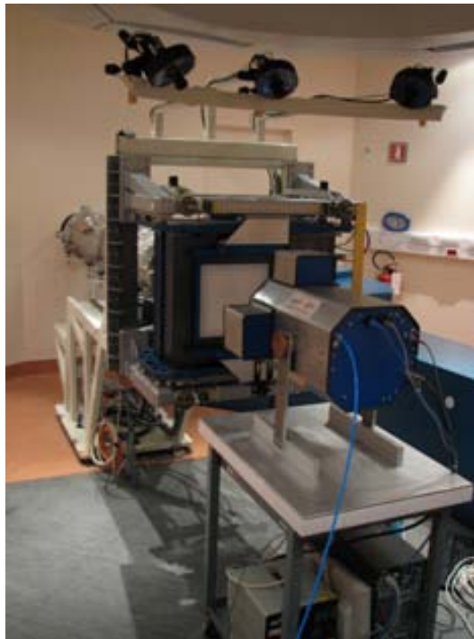
Figure 5.57: The PRR10 in one of the treatment rooms with horizontal beam at CNAO.
