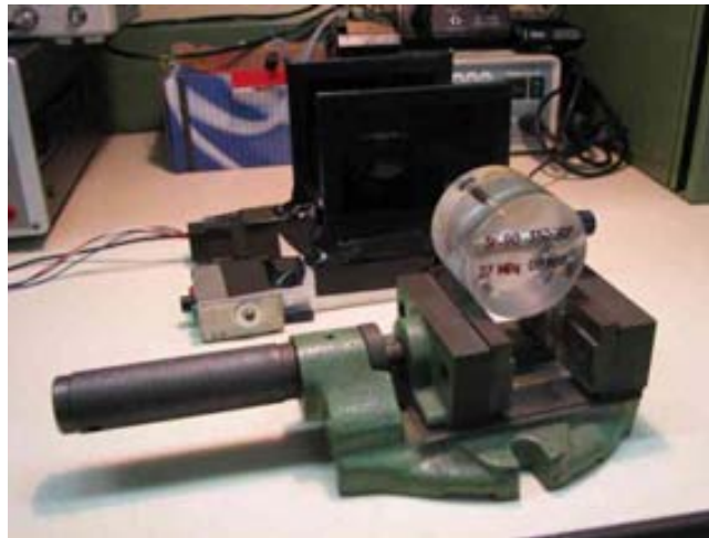
Figure 5.9: Setup for evaluating the response of the scintillator modules to irradiation by a ^{90}\text{Sr} source of electrons. The first module is under test and the second is used for triggering the data acquisition.
