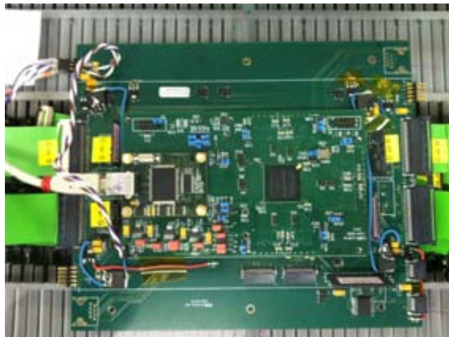
Figure 5.13: The central DAQ for readout of the 30 plastic scintillator modules. The central DAQ holds an FPGA as well as a QuickUSB module and is connected to a mezzanine board which serves as a fan-out for communication with the modules as well as providing the 67 V base voltage needed for the SiPMs.
