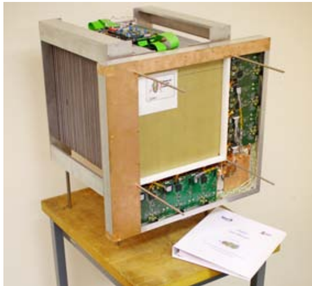
Figure 5.71: The new PRR30 instrument in its current state of development. 48 scintillator modules have been assembled and one GEM detector has been fully equipped and tested with GEMROC front-end electronics.
