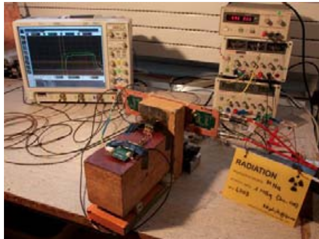
Figure 7.34: Experimental setup for measuring the axial position resolution of the compact MRPC modules. A 3 \times 3 \text{ cm}^2 SiPM and 3 \times 3 \times 20 \text{ cm}^3 LYSO crystal assembly is used to select coincidences. A 5 cm lead block with collimator ensure that only a narrow beam of 511 keV gammas from the ^{22}\text{Na} source are incident on the MRPC detector.
