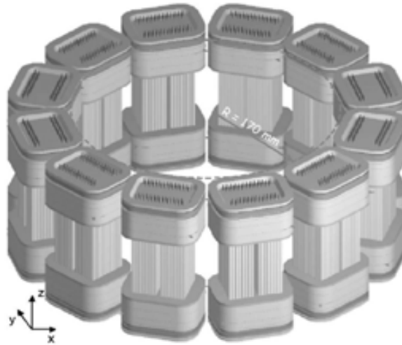
Figure 6.7: A proposed PET design where the DOI information is extracted from the ratio of signals recorded by photodetectors at each end of the crystal.
