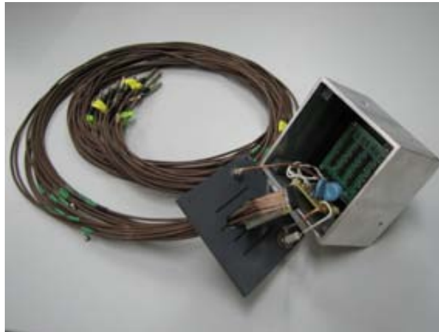
Figure 7.10: The aluminum box assembly opened and showing the rear-panel connection of the HV and MCP-OUT signals and 16 coaxial cables.
