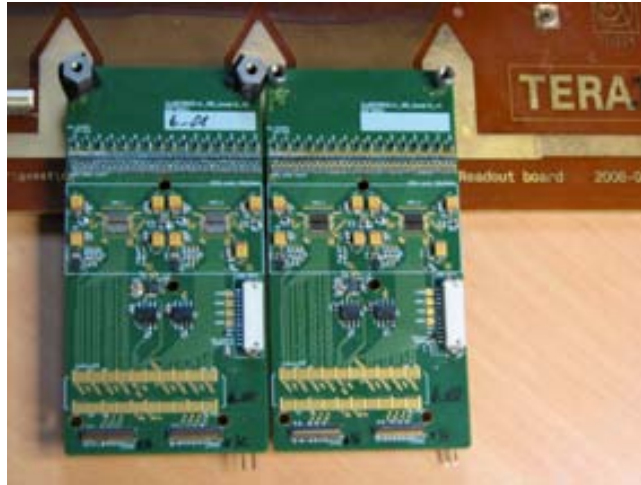
Figure 5.67: GEMROC hybrids mounted on the 30x30 cm 2 GEM readout board. Each hybrid reads 64 channels.
