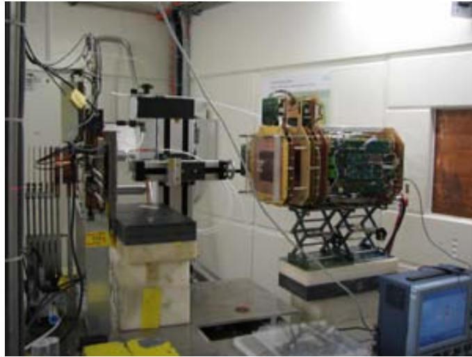
Figure 5.33: The AQUA PRR10 installed in the PSI experimental hall ready for testing with proton beams.
