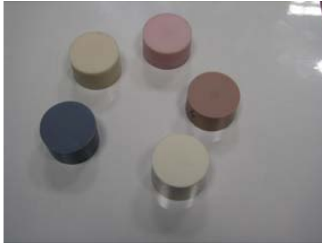
Figure 5.59: Various tissue-equivalent phantoms which have been used in the CNAO beam tests with the PRR10 detector.
