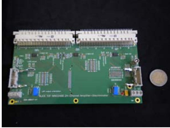
Figure 7.24: The 24-channel NINO card designed for the ALICE experiment and used in our tests.
