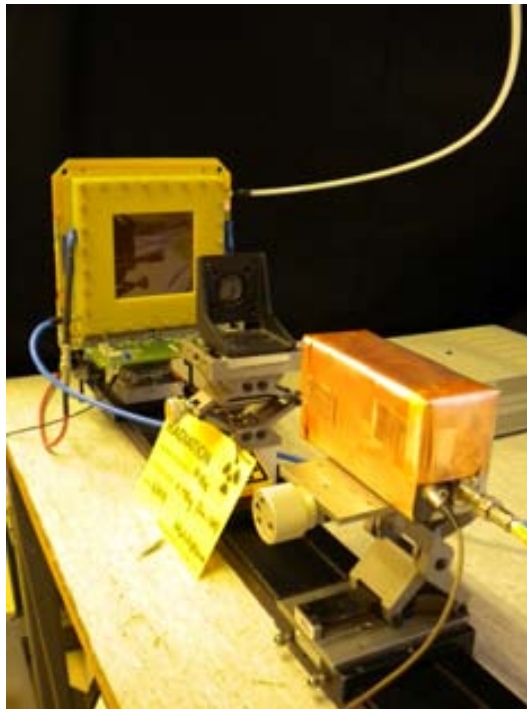
Figure 7.25: Experimental setup for measuring the MRPC efficiency to 511 keV photons. A ^{22}\text{Na} source is placed precisely between the MRPC under test and a BGO-PMT assembly.
