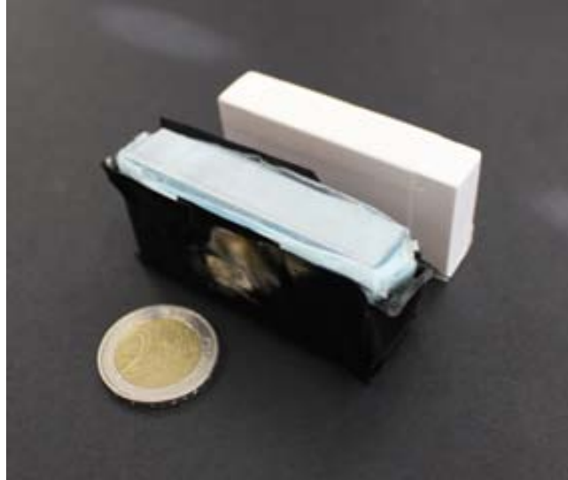
Figure 7.3: Two of the LYSO crystals wrapped in Teflon then black tape for mounting on photo-multiplier.
