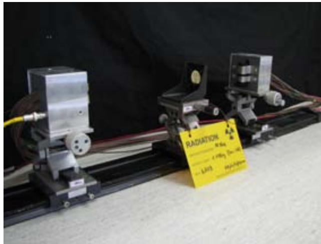
Figure 7.17: Two MCP-PMT modules mounted in a coincidence setup with a ^{22}\text{Na} point source. Only one LYSO crystal is coupled above 16 anodes on each of the modules.
