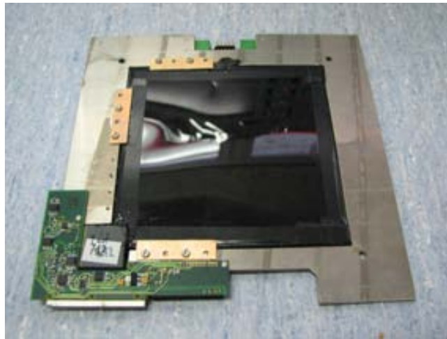
Figure 5.11: A pair of scintillator modules mounted on support frames. The design allows the scintillators and readout electronics to be packed tightly, an important requirement for minimizing the size of the full range telescope.
