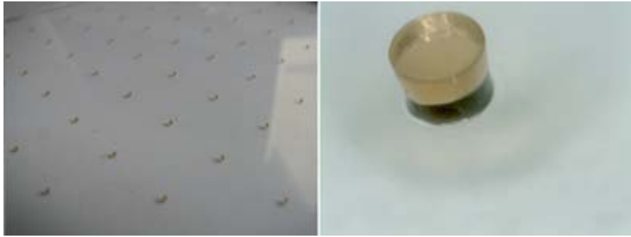
Figure 7.21: Insulating spacers produced from photo-sensitive polyimide patterned on glass. Spacers are 300\ \mu\text{m} in height and 300\ \mu\text{m} diameter.
