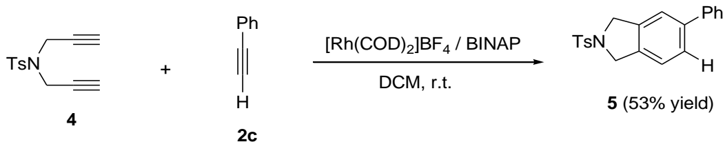
Scheme 4. [2+2+2] Cycloaddition reactions between diyne 4 and phenylacetylene 2c studied by ESI-MS.
