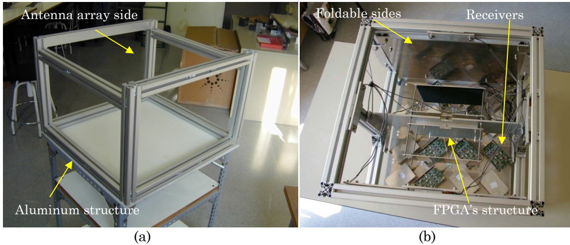
Figure 7.20 PAU-RAD mechanical aluminum structure with a size 110 x 120 x 80 cm, (a) the structure empty, and (b) the structure being mounted, with the empty FPGA's structure in the center.
