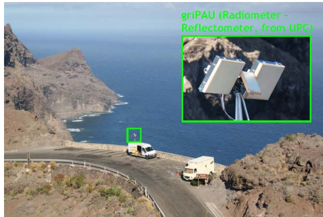
Figure 2.12. griPAU deployed during the ALBATROSS 2009 field experiment [38].
