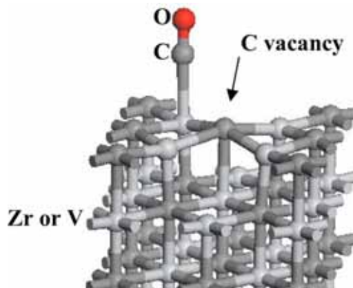
FIG. 10. (Color online) Structure for the formation of CO by reaction of an O adatom with a C atom of the ZrC(001) or VC(001) surface. The O atom is shown as a black (red on the web) sphere. C atoms are represented as dark gray spheres, while light gray spheres denote Zr or V atoms.
