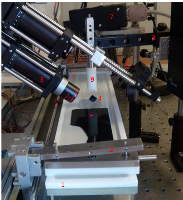
Figure 7. Experimental setup for the transfer of Langmuir monolayers onto a solid substrate by means of the Langmuir-Blodgett technique. (1) custom-made Teflon trough, (2) movable barriers, (3) KSV-Nima Minitrough dipper, (4) silicon substrate ( \text{SiO}_2 SURF Standard, Nanolane) glued to a glass slice, (5) thermistor, (6) filter paper Wilhelmy plate, (7) electrobalance, (8) BAM, (9) dipper clip.
