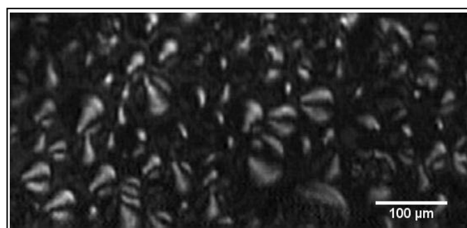
Figure 3. BAM micrograph of a cis-trans 8Az5COOH monolayer doped with a 6% of S-enantiomer, at 20°C and low surface pressure.
