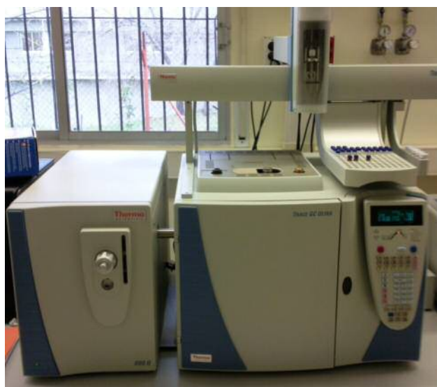
Figura 3.6. GC-MS (Thermo Trace GC Ultra – DSQ II)
