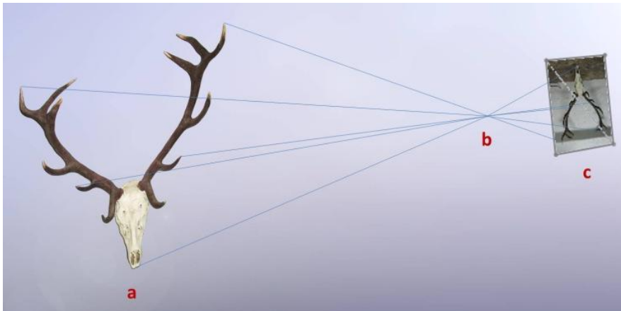
Figure 6.2. Trajectory of the rays of incidence on the plane of a photograph. a) Real object; b) position of the camera lens; and c) photograph.
