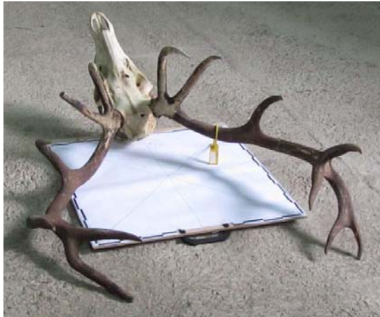
Figure 6.5. Metric reference element of known dimensions (square plate of 50x50 cm).
