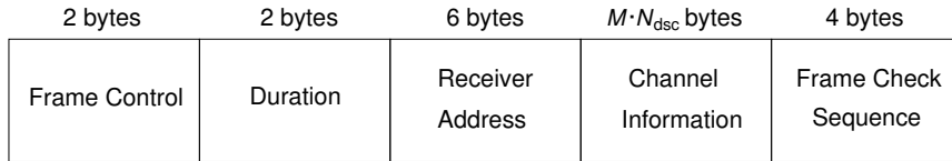
Figure 6.7: Frame Structure of MU-CTS
