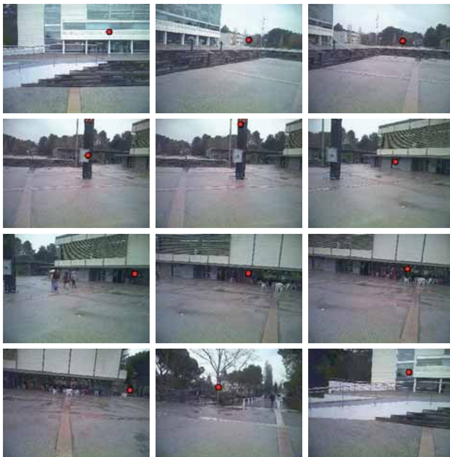
Figure 5.3: A sequence of 12 selected frames taken by the Mobile Eye Tracker's scene camera. Following the frame sequence by rows, from the top left to the bottom right, a typical pattern of a subject making a full 360 degrees scan of the scene while searching for text objects. The FOA position is superimposed in red color.
