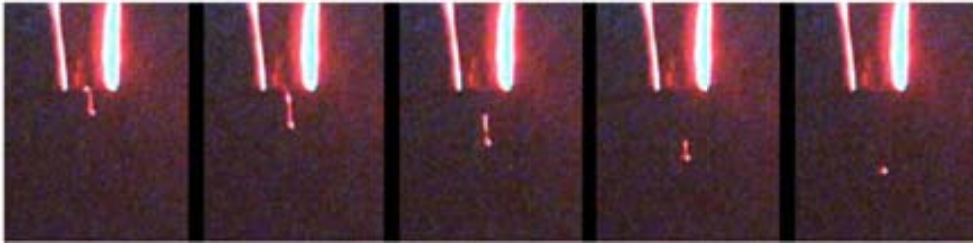
Figure 2.6.: Drop formation sequence of a 0.3M LSMO precursor solution. The solution was printed by using a piezohead with a nozzle orifice of 60\mu\text{m} with voltage amplitude V_1 = +25\text{V} ; V_2 = -20\text{V} ; corresponding times t_{\text{rise}} \sim 3\mu\text{s} ; t_{\text{dwell}} \sim 11\mu\text{s} ; t_{\text{fall}} \sim 3\mu\text{s} ; t_{\text{echo}} \sim 11\mu\text{s} ; t_{\text{final rise}} \sim 2\mu\text{s} and frequency f = 100\text{Hz} .
