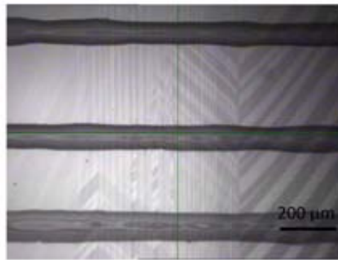
Figure 5.22.: Effect of ink-jetted tracks quality on substrate temperature. YBCO precursor tracks after 2 depositions using 2 nozzles of the printer set-up. Drop pitch, substrate temperature and cartridge temperature were fixed at 20 \mu\text{m} , 45°C and RT respectively. In this case, track width increases from 75 \mu\text{m} to 120 \mu\text{m} .
