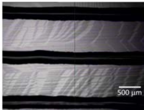
Figure 5.19.: YBCO precursor tracks after 2 depositions using 2 nozzles. Drop pitch, substrate temperature and cartridge temperature were set at 5\mu m , 30^\circ C and RT, respectively.
