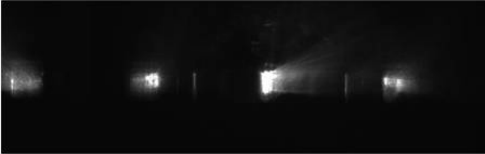
Figure 4.8: Complete picture of intensity profile at 1x4 BS output.
