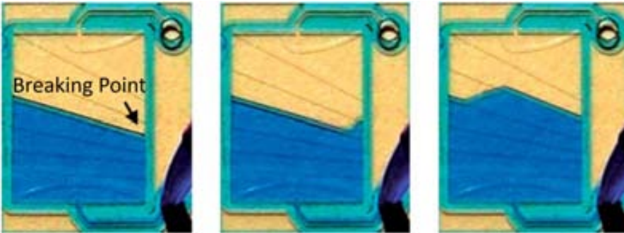
Figure 2.8: A diagonal phaseguide to produce controlled overflow in an specific region.
