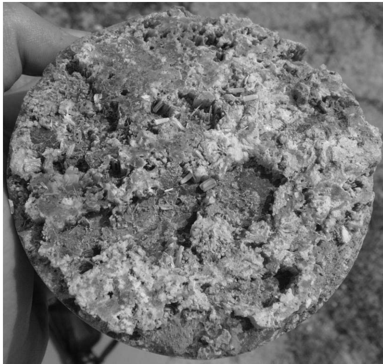
Figure 7.4. Gypsum crystal growth in needles in a recovered core from a borehole drilled for hydraulic cross-hole tests, at depths corresponding to the active layer. Gypsum crystals form needles partially filling the open vein
