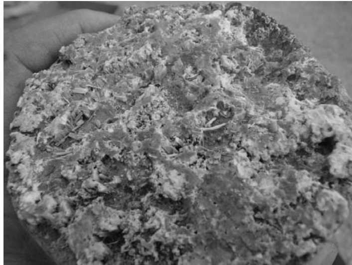
Figure 4.24. Crystals in a core from a Cross-hole borehole
