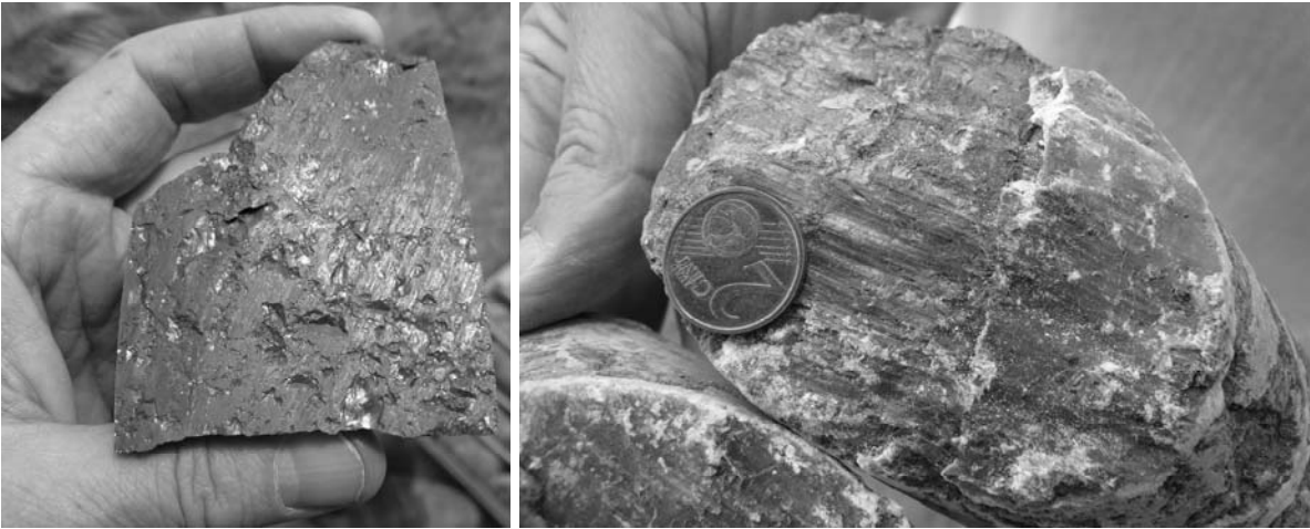
Figure 5.6. Striated discontinuities found in cores recovered in borehole B1 at depths below the elevation of Lilla tunnel invert
