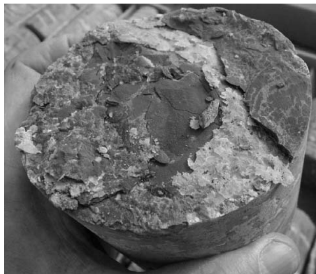
Figure 4.21. Laminar gypsum crystal growth developing inside the clay matrix. Observations in a recovered core from a borehole tested during hydraulic cross-hole testing at depths corresponding with active layer
