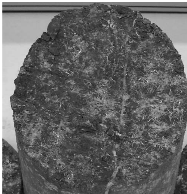
Figure 3.9. Thin gypsum needles observed in a claystone discontinuity in a core recovered from depth 4.2 m at chainage 411 + 600
