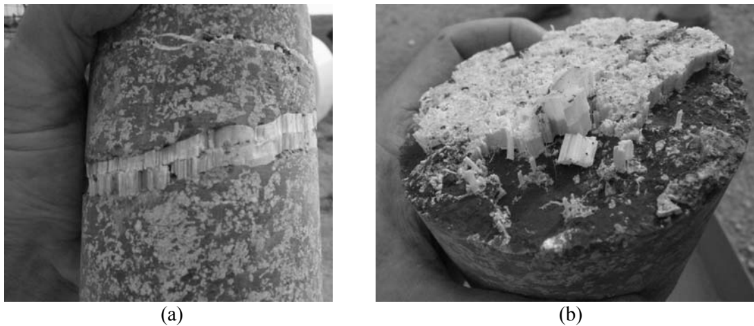
Figure 4.20. Gypsum crystal growth in needles. Observations in a recovered core from a borehole drilled for hydraulic cross-hole testing at depths corresponding with active layer: (a) image of a gypsum filled vein before opening it; (b) Gypsum crystals form needles partially filling the open vein, once it is opened by hand
