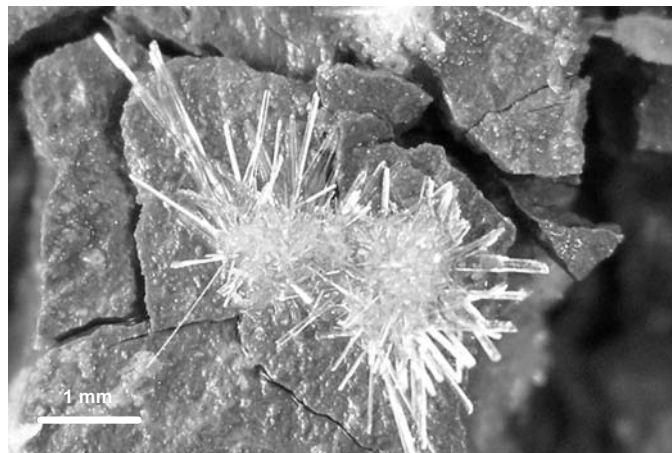
Figure 6.4. Detail of gypsum crystal “rosettes” developing in a discontinuity
