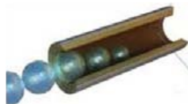
Fig. 4.3.2 Schematic view on the bubble creation inside a microtube, image from Sanchez 2010 #250
