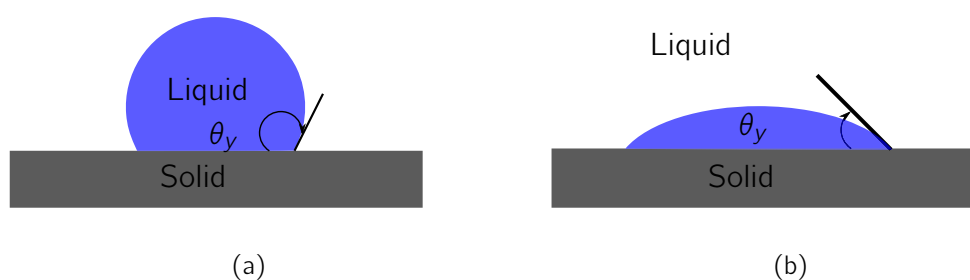
Figure B.1 Difference in wettability. (a) a hydrophobic surface, and (b) a hydrophilic surface.
