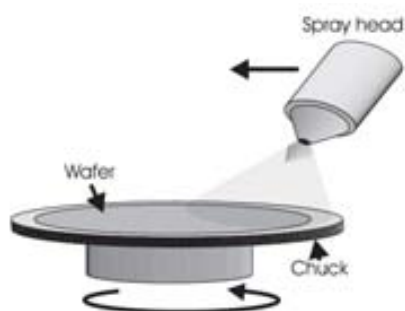
Figure 1.16 Spray coating scheme. Image from www.elve-ow.com
