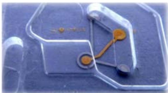
Fig. 3. Electrochemical sensor with gold working electrode and platinum reference and counter electrodes, integrated in the labcard.
