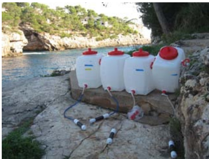
Figure 2.1. Extraction of Ra isotopes from the water sample by gravity filtration through a cartridge loaded with Mn-fiber.
