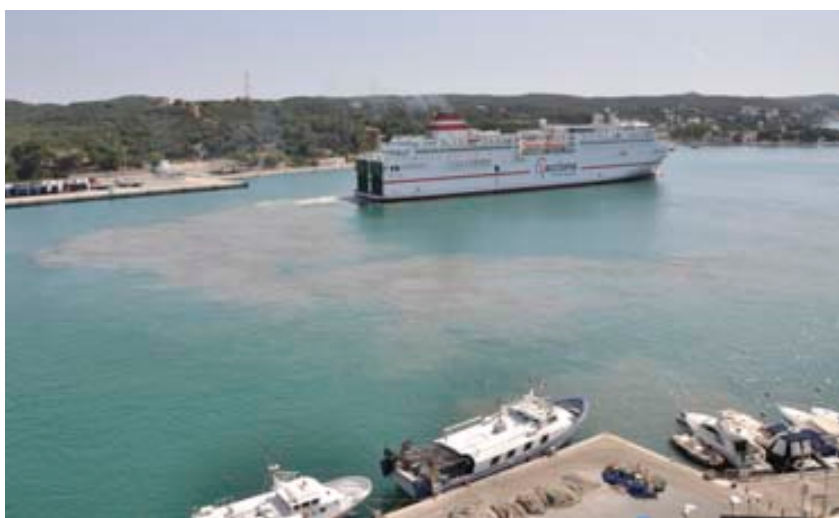
Figure 4.4. Resuspension of sediments produced by the undocking maneuver of a vessel (draft ~6 m) departing from the Port of Maó.
