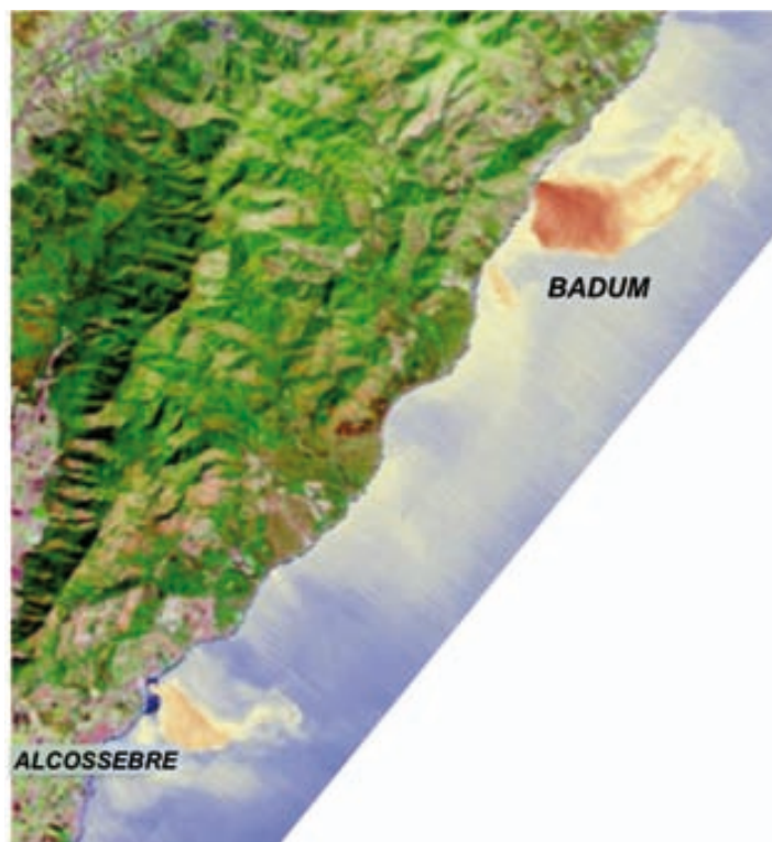
Figure 1.9. Airborne thermal infrared image (TIR) capturing karstic groundwater springs (Alcossebre and Badum springs) discharging to the Mediterranean Sea from the deep aquifer of El Maestrat (Castelló, Spain) (adapted from Garcia-Solsona et al. 2010b).
