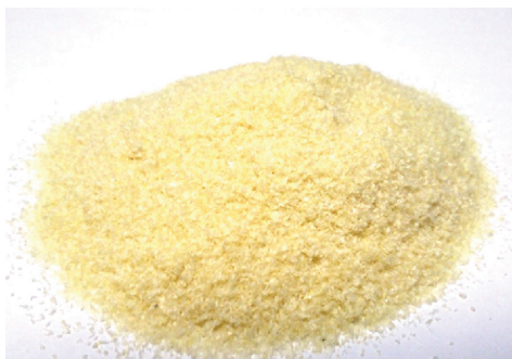
Figure 3.1. Chitosan flakes (particle size G2 < 250 \mu\text{m} ) provided by Aber Technologies (France).
